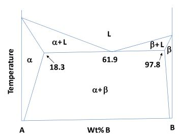
Upon complete solidification of a binary alloy system A-B, the fraction of pro-eutectic  $\alpha$ -phase present is 0.50. The alloy composition in terms of wt%. B is \_\_\_\_\_
